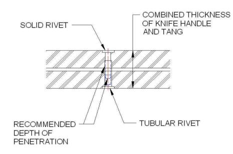
Each unit when swedged together should equal at least 3/4 of the combined thickness of both sides of the knife handle, including the tang. This permits approximately 1/4 of the shank length of the solid rivet and 1/4 of the shank length of the tubular section to extend through the opposite side of the tang.
